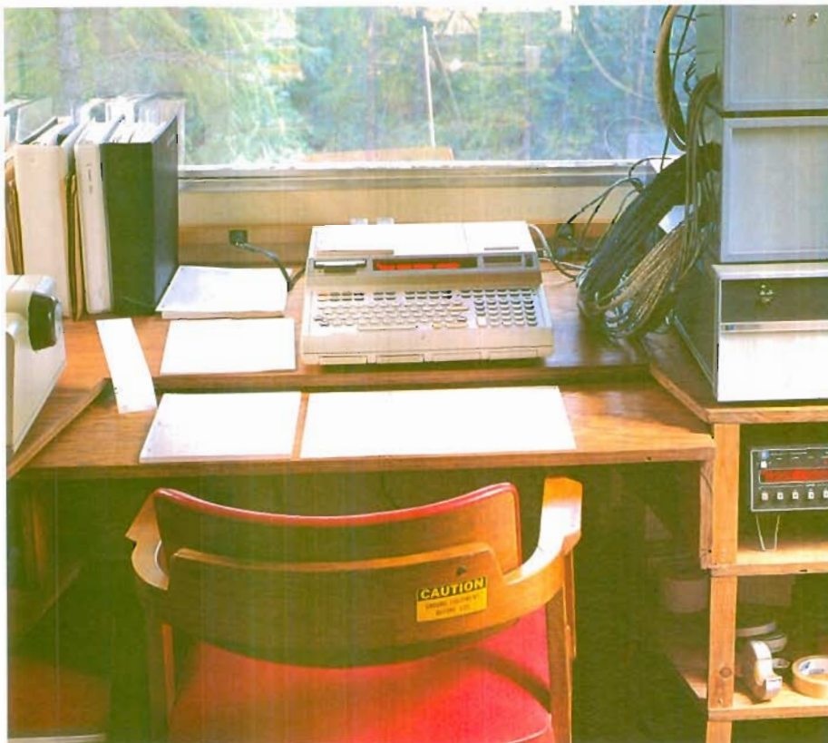
Control of the cuvettes, as well as data collection from instrumentation on the platforms, centers on the 9825A system located in a trailer overlooking the experimental forest.
