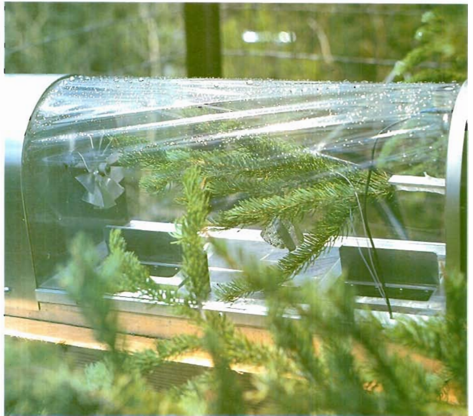
One branch from a conifer at the test site set up by Dr. Kaufmann is isolated inside this chamber, or cuvette. Periodic measurement cycles determine the amount of water the branch transpires.
